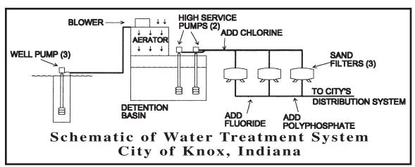
pumps, called high service pumps, move the water from the detention basin through pressure sand filters completing the iron removal process. Chlorine is added prior to the pressure sand filters for disinfection. The water leaving the filters enters the water distribution system after receiving fluoride and polyphosphate addition and flows to the homes, businesses and industries of Knox.
